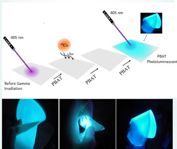
**Fig. 5** Schematic drawing of radio-induced tunable photoluminescence in PBAT copolymers
