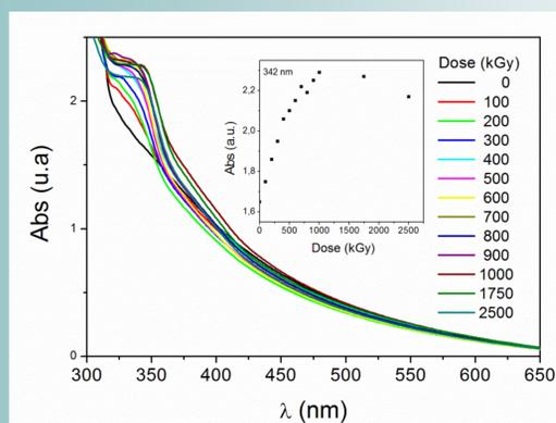
**Fig. 1** UV-Vis absorbance spectra for PBAT copolymers irradiated with gamma doses. The inset shows the absorbance intensity at 342 nm as a function of gamma dose.
