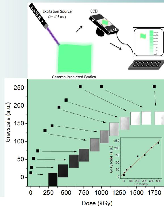
**Fig. 3** Grayscale from 0 to 255 images using the camera from Hamamatsu PBAT films irradiated with different doses of gamma radiation
