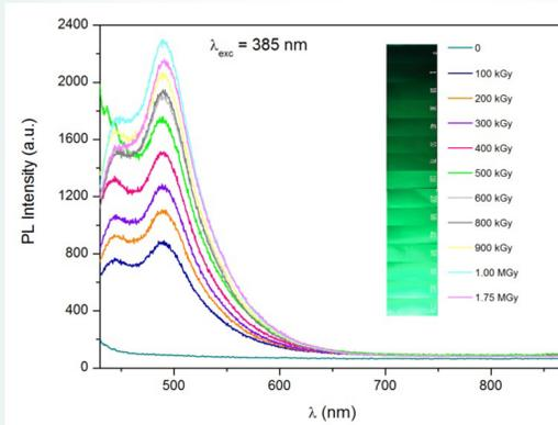
**Fig. 2** Photo-stimulated luminescent emission spectra of PBAT excited with LED source at 385 nm, for doses ranging from 0.0 to 1.75 MGy. The Corresponding photos taken during excitation vary from dark green (0.0 kGy) to very bright green (1.75 MGy), for increasing doses.
