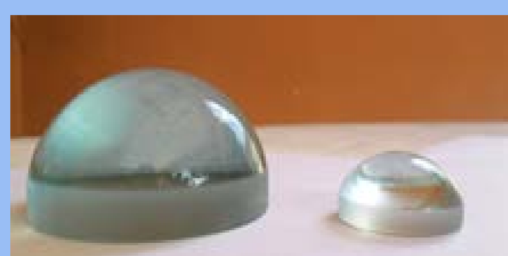
Figure 2. Converging lenses, with 60.0 cm (left) and 32.0 cm (right) of diameter.
