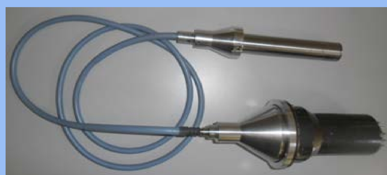
Figure 1. Prototype developed - photomultiplier coupled with a NaI(Tl) detector using a remote probe of optical fiber.
