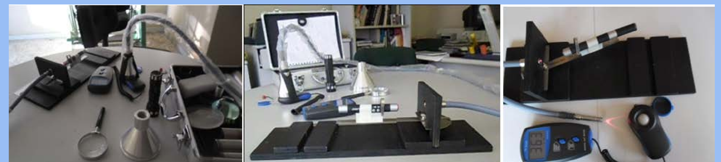
Fig 4. Device for measuring of the fiber acceptance angle using a laser light and a compact size digital lux meter (MLM-1011) Minipa, measuring range from 1 up to 100000 lux.
