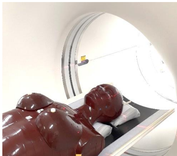
Fig. 2. Positioning of the Alderson female phantom in the gantry.
