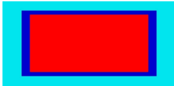
Fig. 4. Homogeneous fuel plate cross-section, image generated by SCALE 6.0
