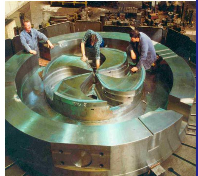
Machining of an IBA cyclotron magnet
