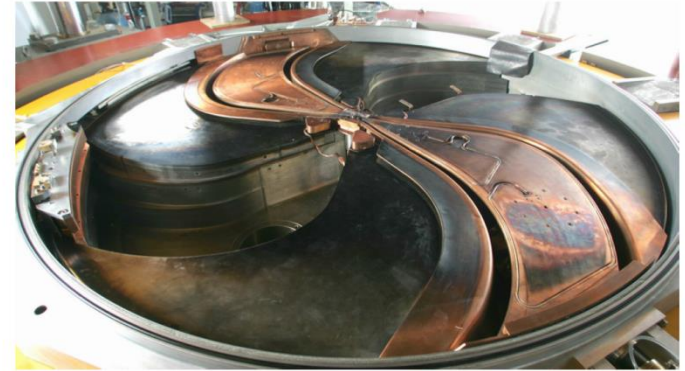
Machining of an IBA cyclotron magnet
