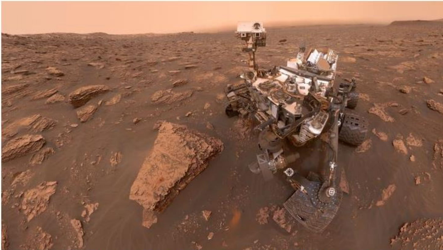
NASA's Curiosity rover is powered by a ^{238}\text{Pu} RTG, meaning it can continue to operate under intense Martian dust storms. ESA is looking to develop RTGs based on ^{241}\text{Am} (Image: NASA-JPL-Caltech-MSSSS)
