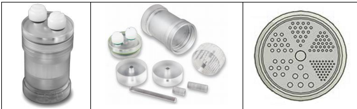
Fig. 2. Left: HotRod Phantom; Center: Details of Phantom components; Right: Upper view of the disc with fillable channels arranged into six groups of different diameters [4].
