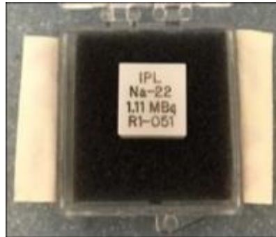
Fig. 3. ^{22}\text{Na} point source [4]. Source: Author archive.
