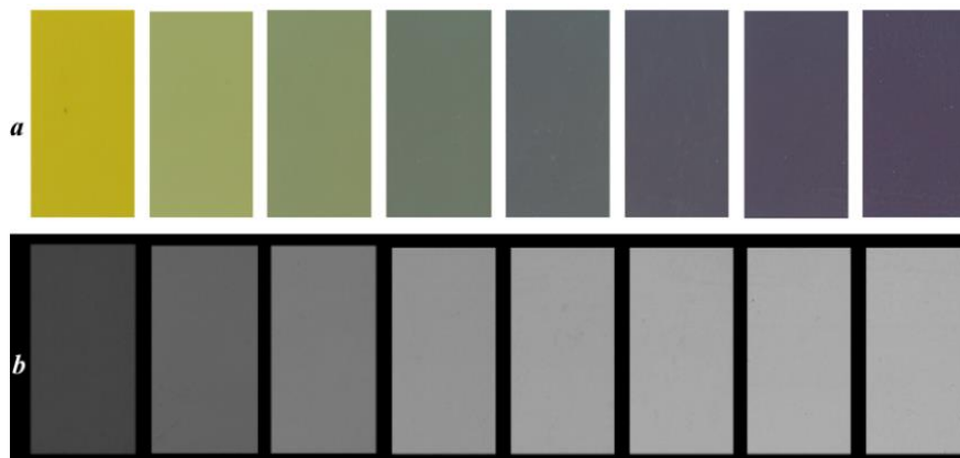
Fig. 3. Images of the strip of the EBT3 film. Before exposure (a), after exposure (b), red channel
