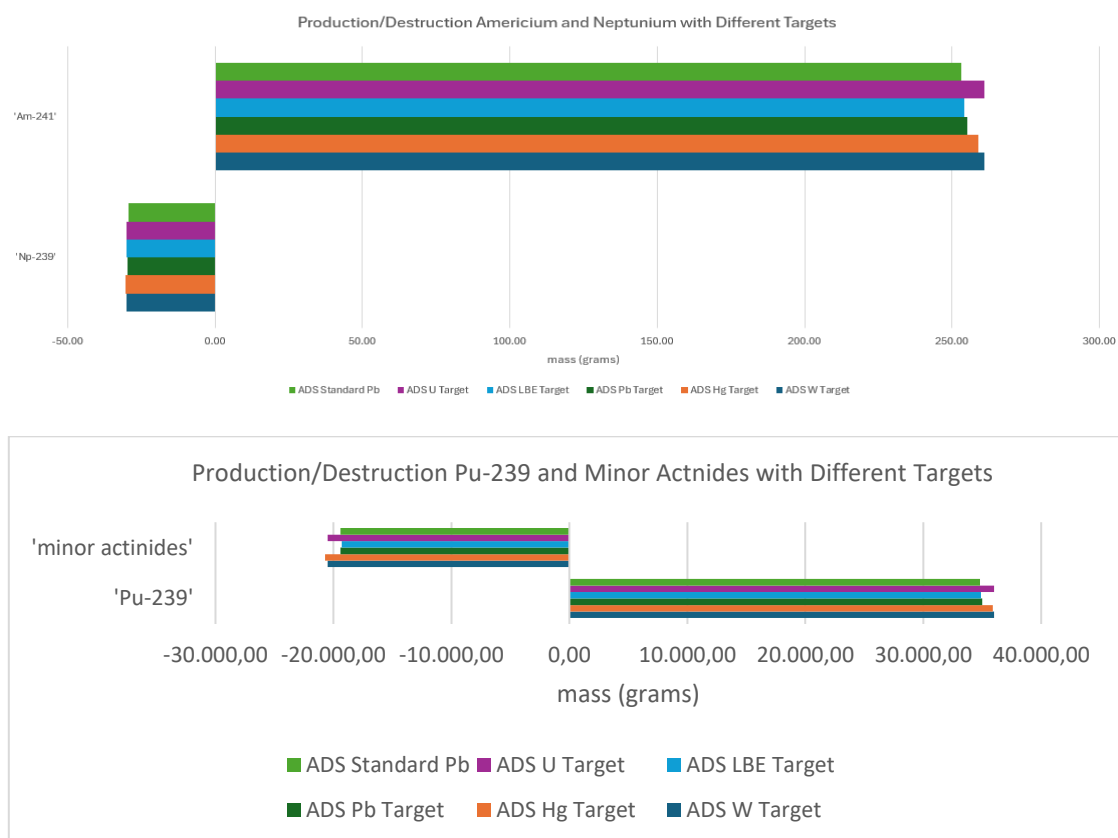
Fig 4. Behavior of (a) total actinides, (b) and tree specific isotopes: Pa-231, Np 239 e Pu-239 produced or destroyed in ADS reactor with different targets.
